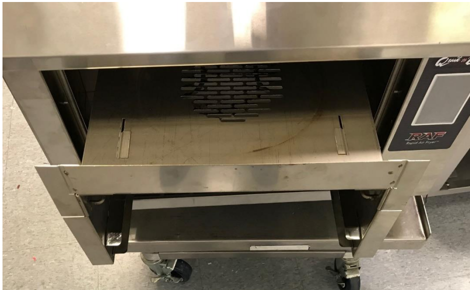
Air Plenum Pulled Out of the RAF
