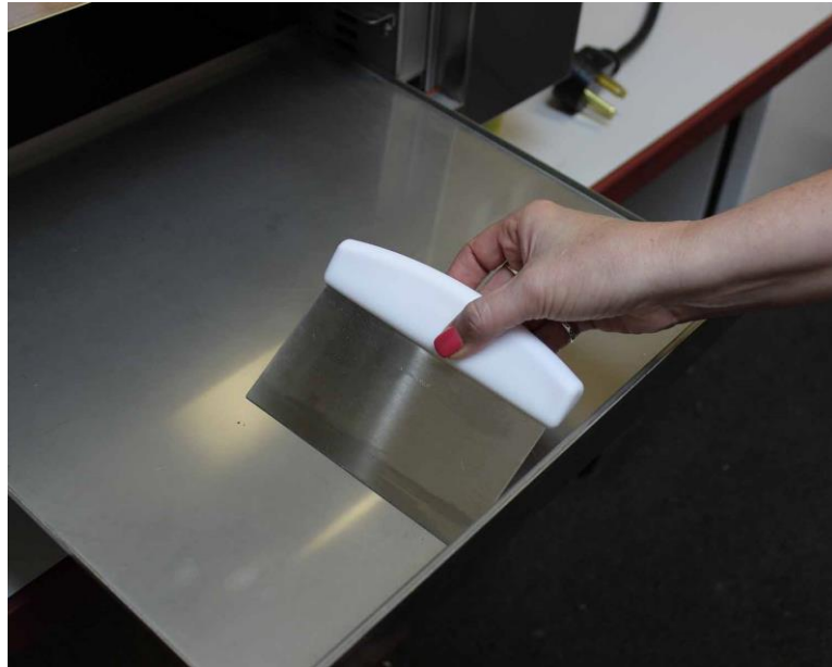
Scraping the Drip Tray to Clean
